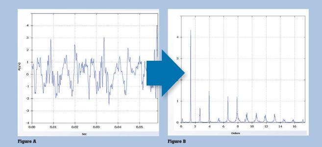
domain data is used to calculate one single overall vibration value. This single value can be used as an indicator of the overall health of the machine. (Note: there are multiple methods available for calculating the overall vibration value. They are described in the appendix for the interested reader). The benefit of overall vibration analysis is its simplicity – there is only one number to examine. However, there are three limitations of using overall vibration analysis that are worth noting:
