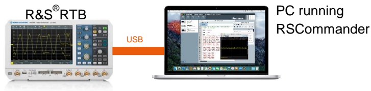
Figure 2: USB instrument connected to PC
