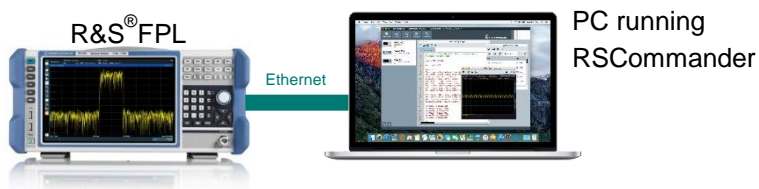
Figure 3: LAN instruments connected to PC
