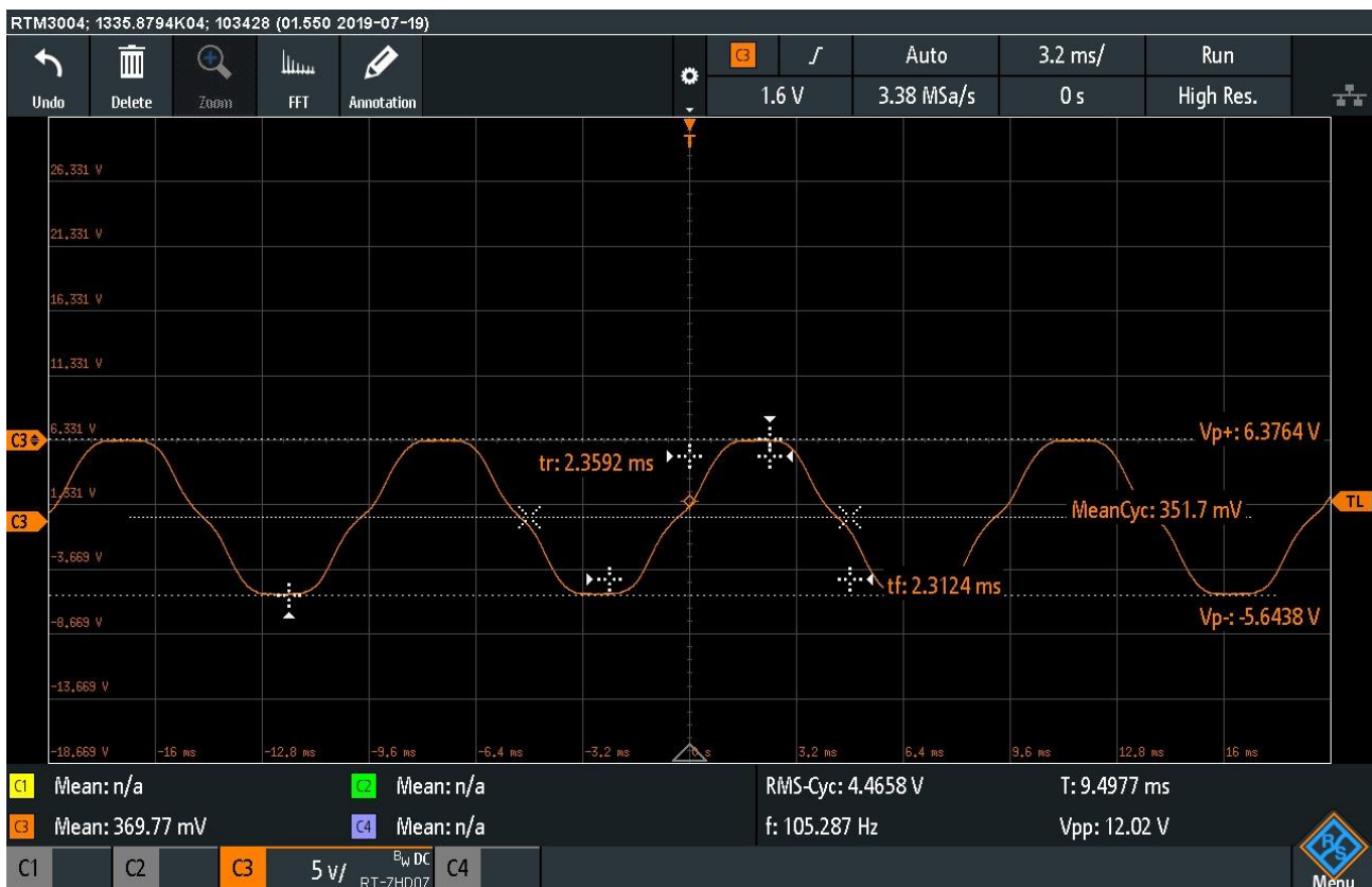
Figure 3-4: Trapezoidal Back EMF measured in one Phase of the BLDC motor.
