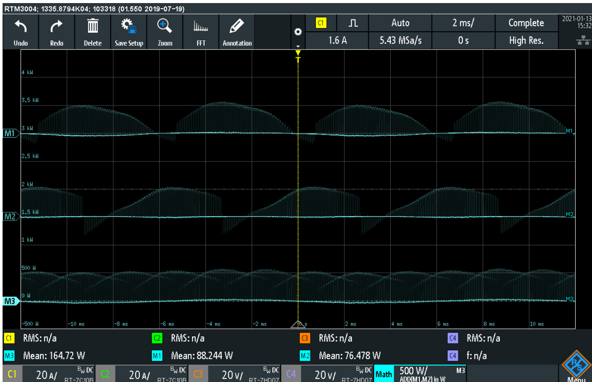
Figure 7-4: Math Waveforms based on Voltage and Current Measurements on Ch1 - Ch4.
