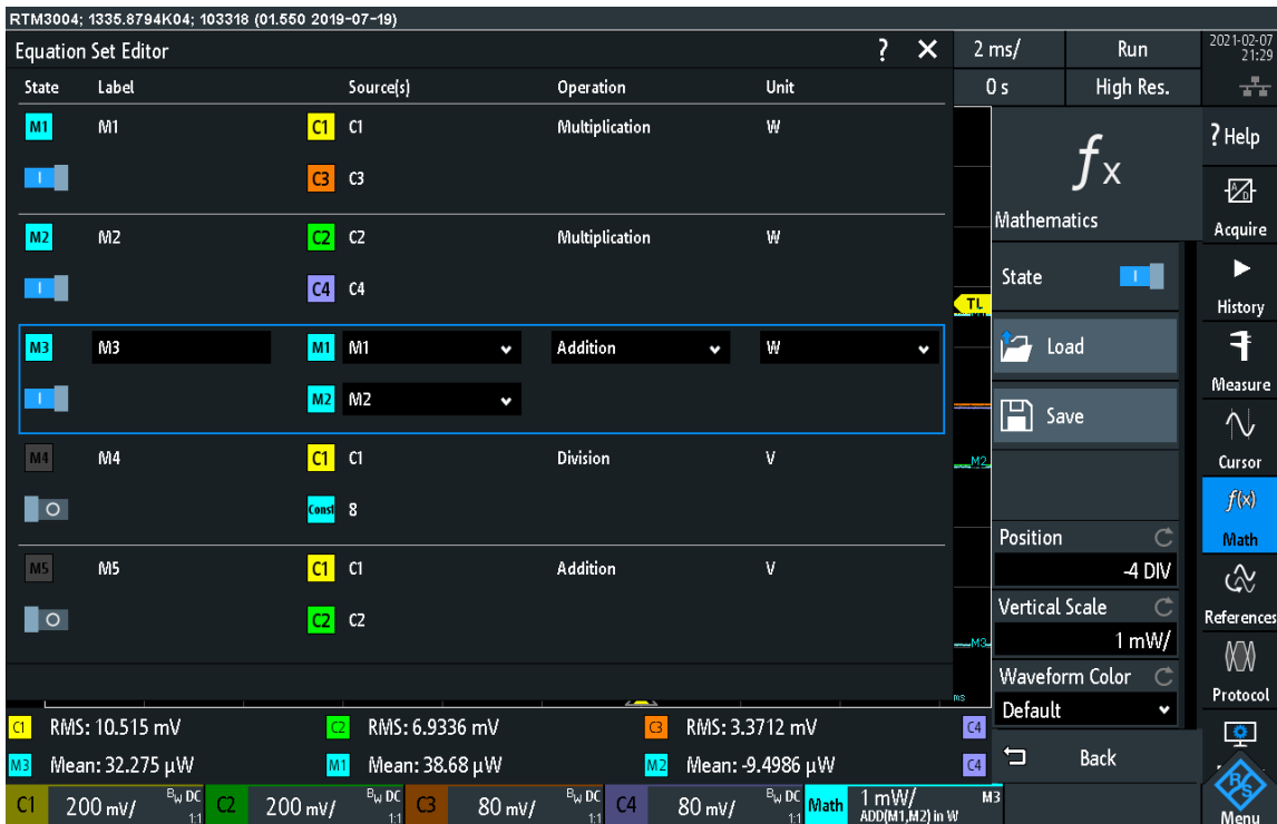
Figure 7-3: Math Equation Editor Configured for the Two-Wattmeter Power Measurement Method.
