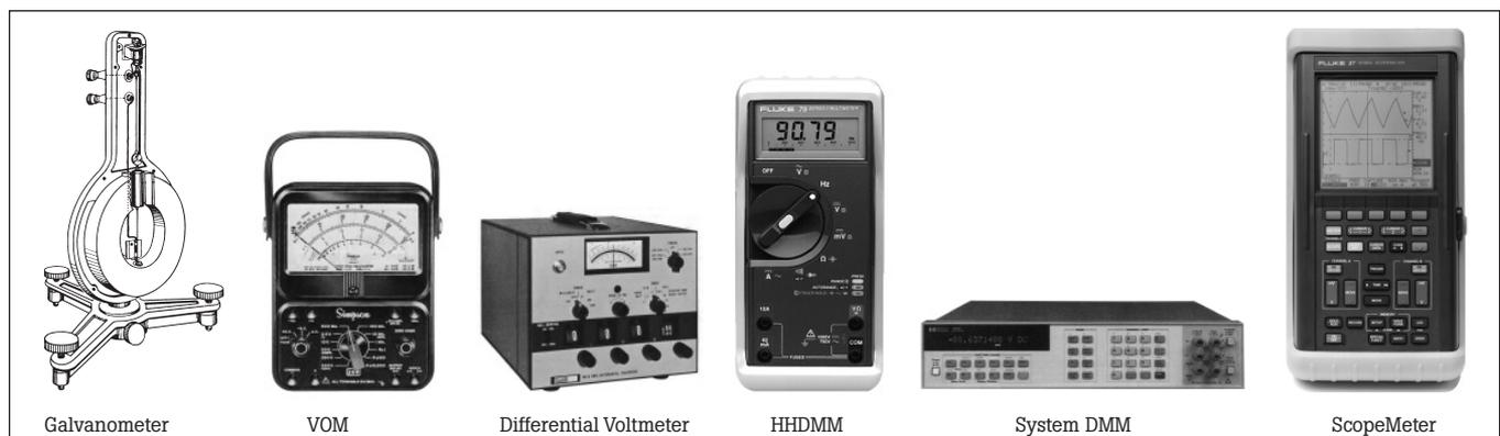
Figure 3. Examples of increasing functionality in electronic test tools.
