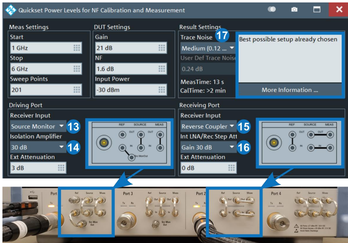
Figure 4-5: Proposed R&S®ZNA hardware settings in the quickset dialog
