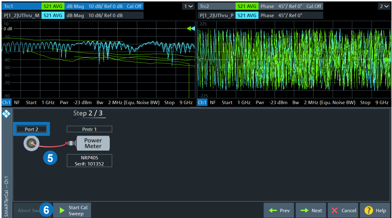
Figure 4-9: Power calibration of the noise figure channel
