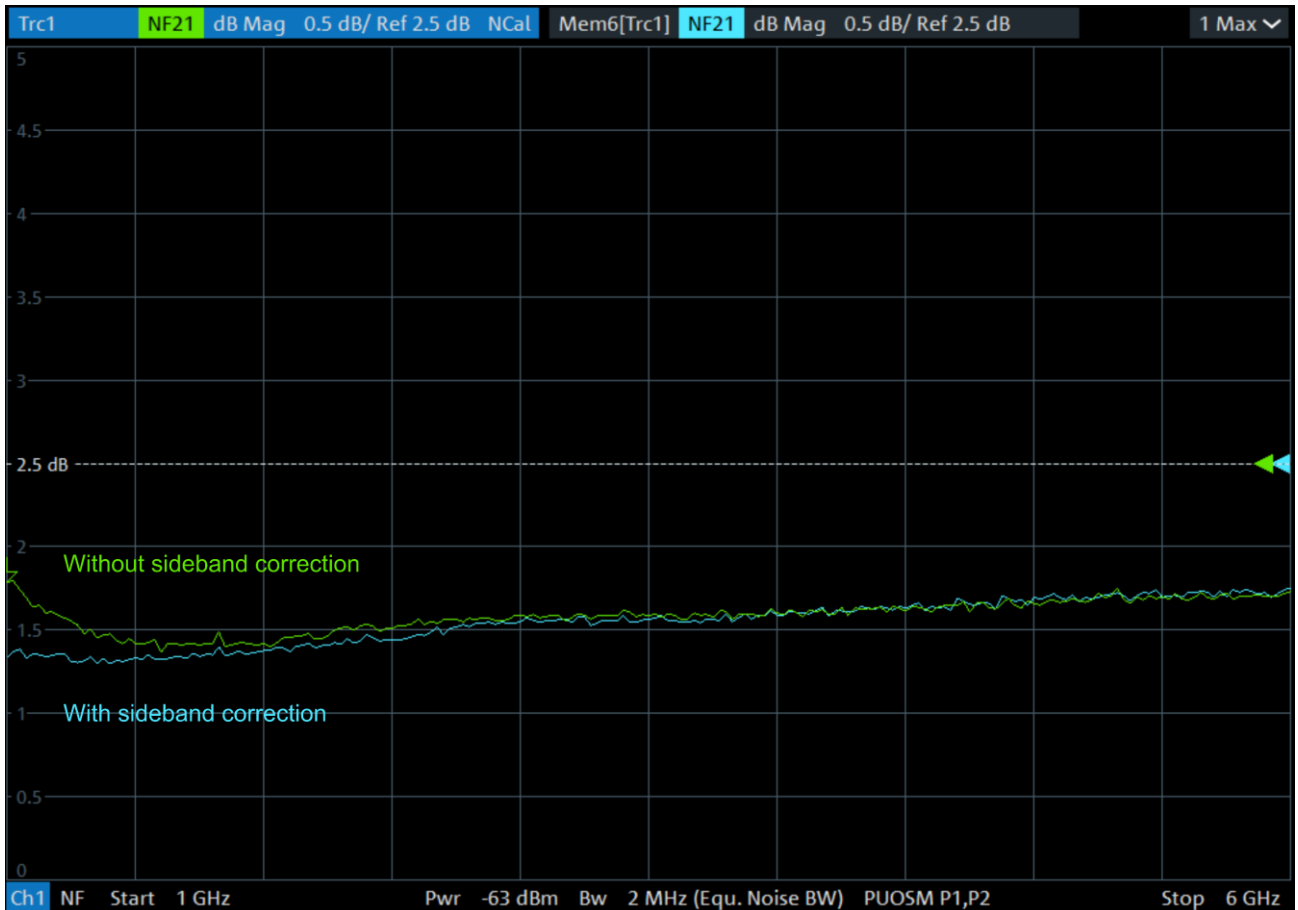
Figure 4-17: Comparison of NF with and without sideband correction
