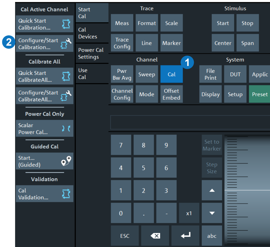
Figure 4-6: Start NF calibration
