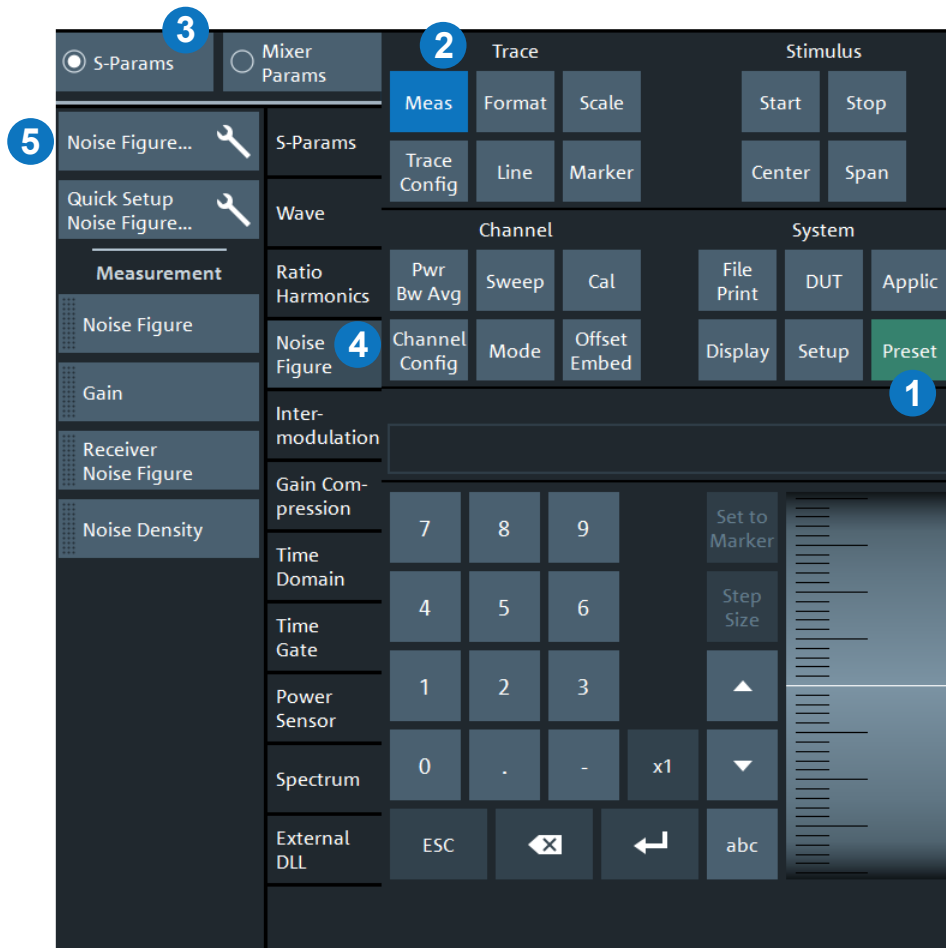
Figure 4-2: Configure a noise figure channel
