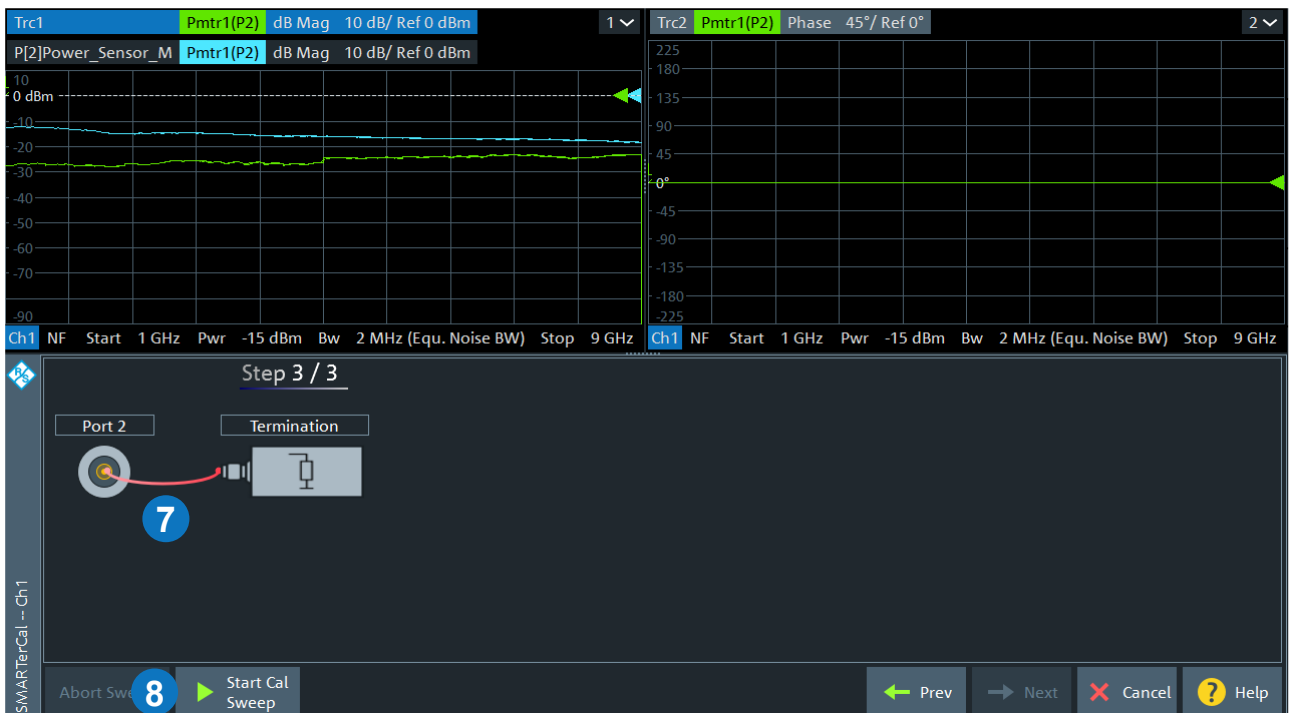
Figure 4-10: Receiver noise calibration of the noise figure channel
