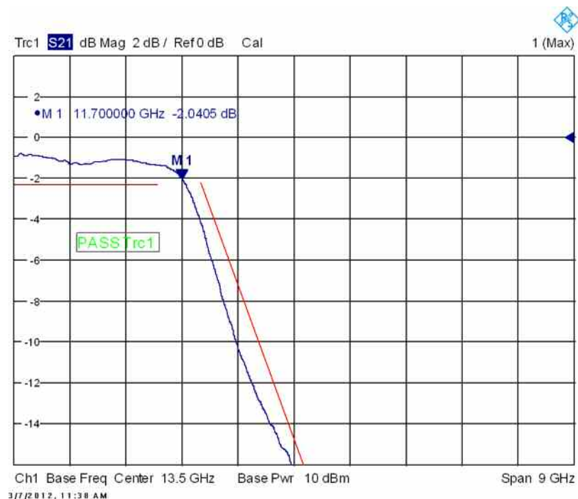
Figure 30: radar X-band lowpass filter transfer characteristic with limit lines
