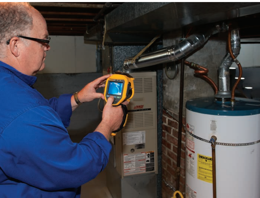
An infrared camera can detect where is it wet and where is it not wet.
