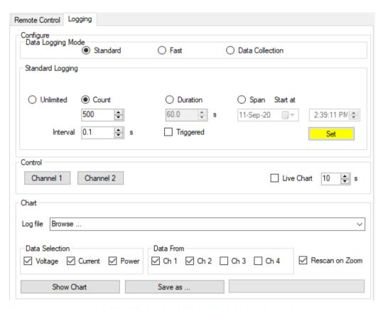
Fig. 4-4: Logging tab of the NGM & NGL Logging & Charting Tool with standard logging
